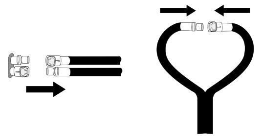
The pressure in the two sets of cells will equalise and the patient will continue to be supported (with the overlay static) for up to 60 minutes with the patient in the supine (lying) position.
