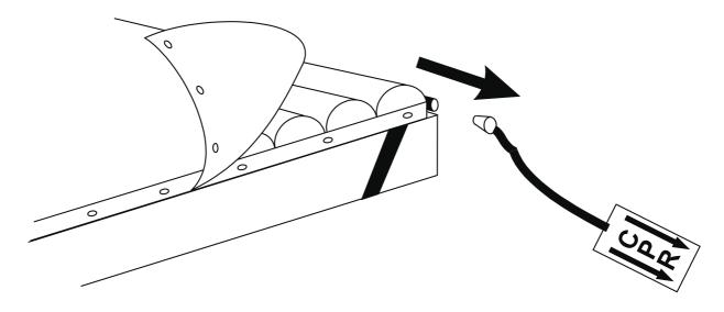
To reinflate the overlay, simply replace the stopper securely, locking connectors onto the manifold and ensuring secure connection of the overlay to the pump.
